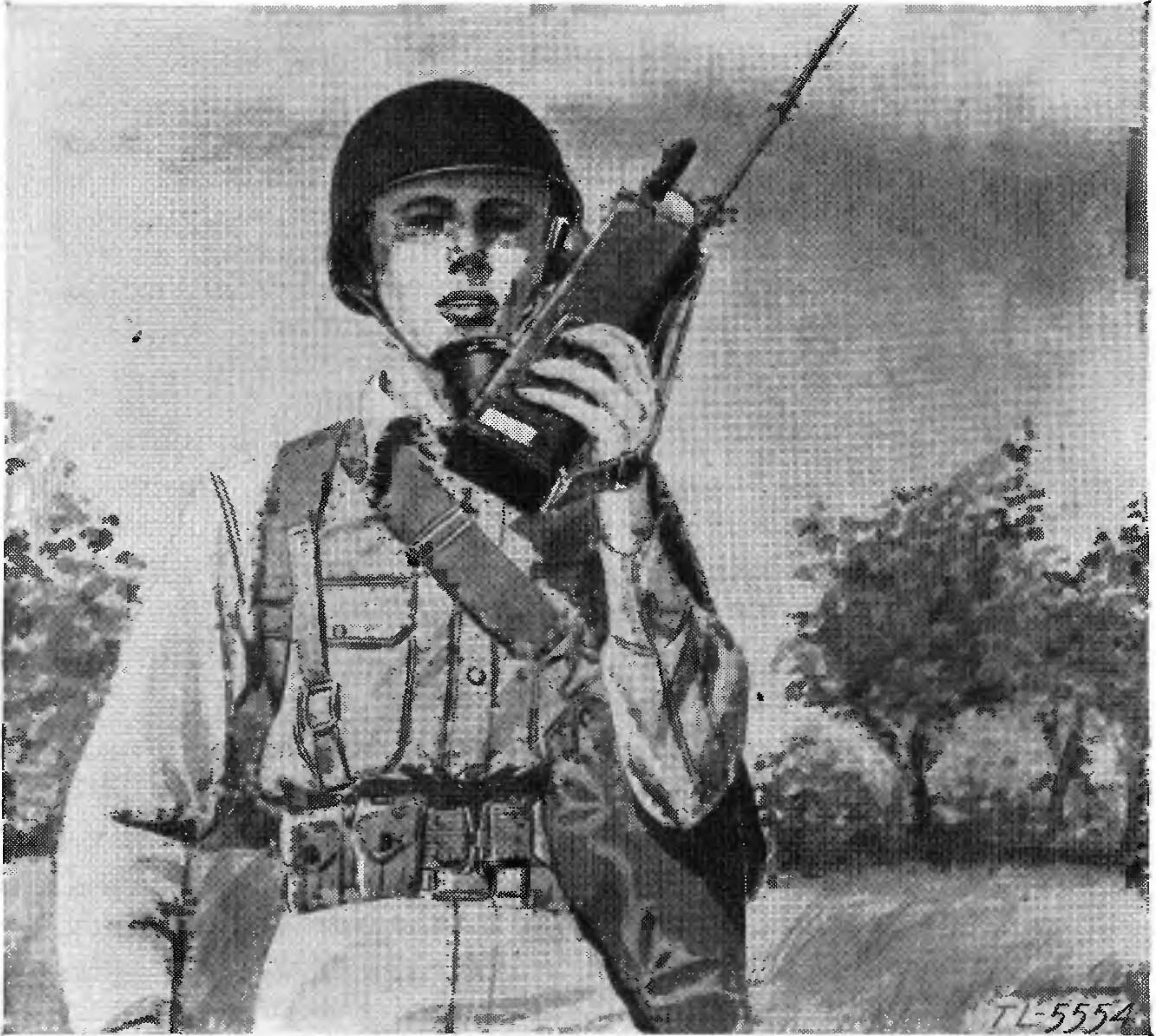
FIGURE 2.—Radio set SCR-536-(*)—in operating position.
